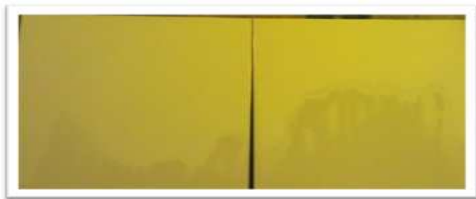
Figure 6. Status surface of plate after dried in 9 minutes. Left: Ra 0.47\mu\text{m} , Right: Ra 0.67\mu\text{m} .
