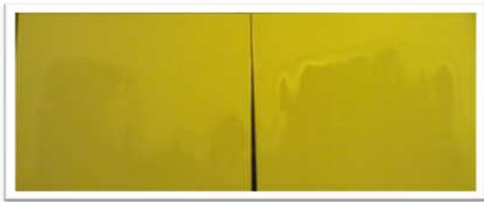
Figure 5. Status surface of plate after dried in 8 minutes. Left: Ra 0.47\mu\text{m} , Right: Ra 0.67\mu\text{m}
