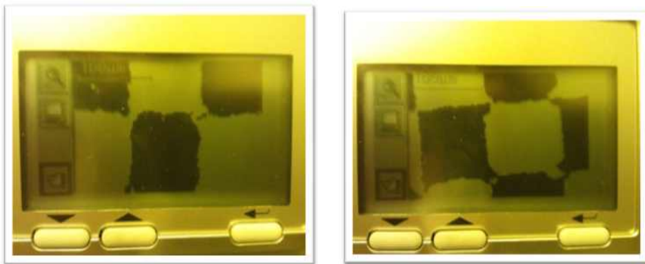
Figure 8. Status 50% dot on the surface of plate. Left: Ra 0.30\mu\text{m} , Right: Ra 0.54\mu\text{m} .
