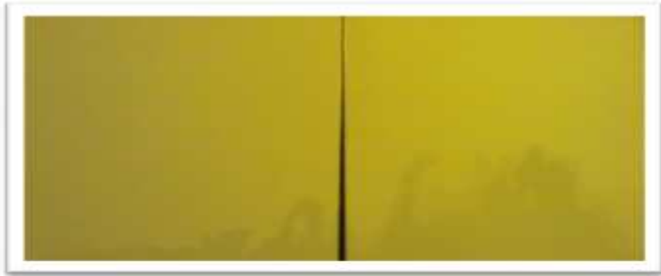
Figure 7. Status surface of plate after dried in 10 minutes. Left: Ra 0.47\mu\text{m} , Right: Ra 0.67\mu\text{m} .
