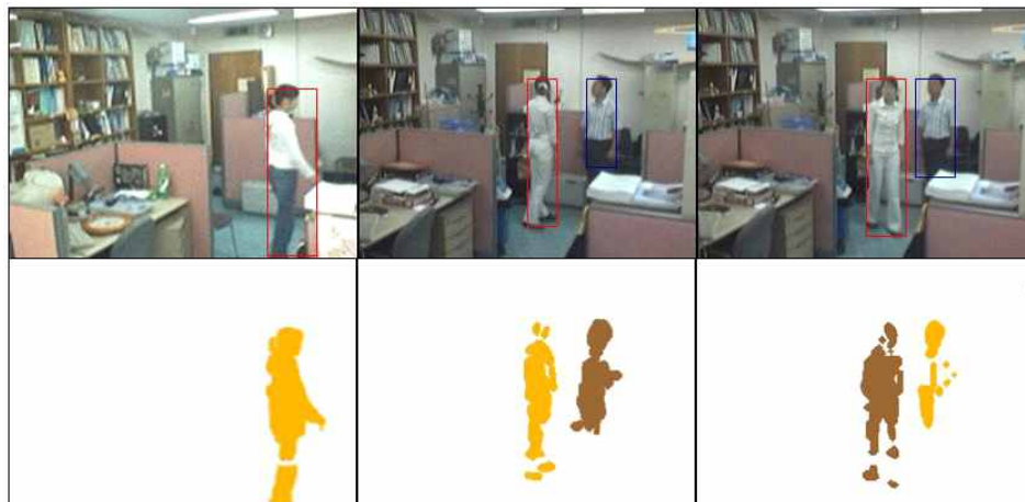
(Fig. 7) The result of object classification
