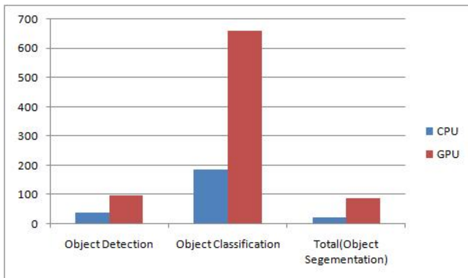
(Fig. 8)Performance evaluation results (unit:frame/sec.)
