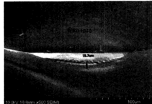
Fig. 8 SEM photograph of tool wear in ultra-precision turning
