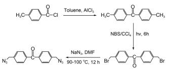
Scheme 1. Synthesis of 4,4'-bis(azidomethyl) diphenyl ketone compound.
