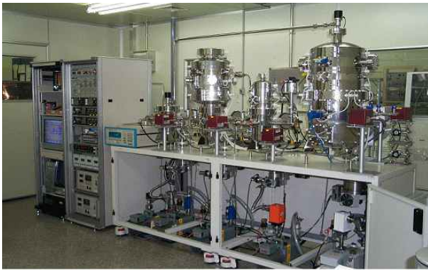
Figure 5. Photograph of the static expansion system. Difference volume chambers are on the right side, and measurement instrument indicators and personal computer are on the left side.
