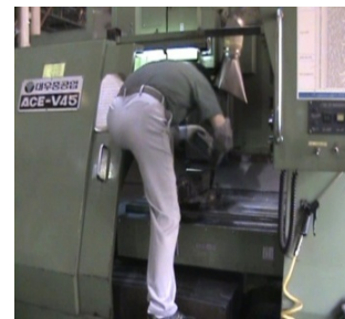
Figure 6. Postures that increase workload on the back which may lead to chronic back pain 2
