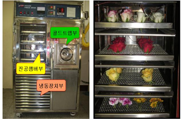
Fig. 2 Photograph of experimental apparatus.
