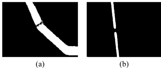
Fig. 8. Detections of short circuit defects.
