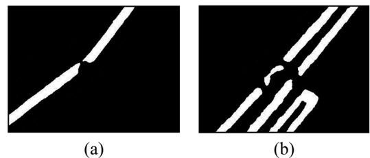
Fig. 6. Detections of open circuit defects.
