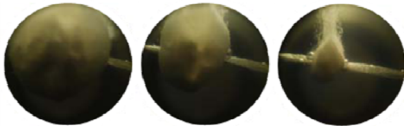
(b) Water flow rate Q_w = 3.87 l/min : t_f = 263 s
