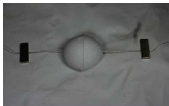
Fig. 4 Hydrate pellet(d=50mm) with string and magnet attached
