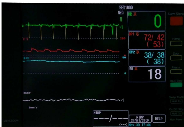
Fig. 4 ECG and aortic pressure measured by patient monitor(HR-500, Fukudadenshi, Japan)
