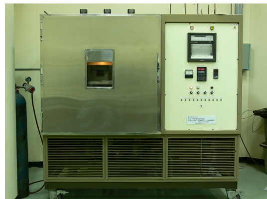
Photo 5 Accelerated carbonation test
