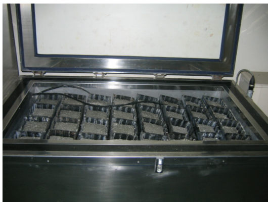
Photo 4 Specimens for freeze-thaw test
