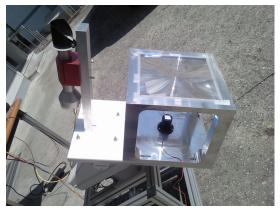
Figure 2: Fresnel lens performance test
