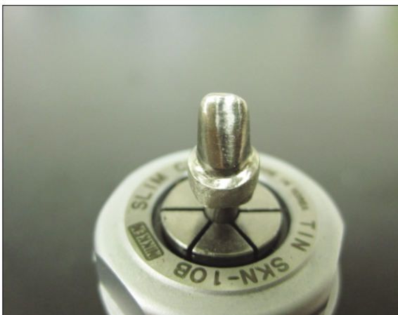
Fig. 1. Metal die used for the fracture strength test.
