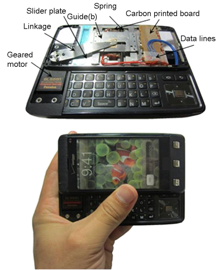
Figure 4. Internal view(high) and appearance(low) of the VSSD
