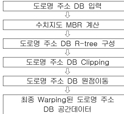
Figure 10. Auto warping algorithm
