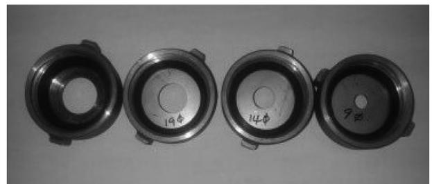
**Figure 2.** Reducing orifices of inner hydrant.
