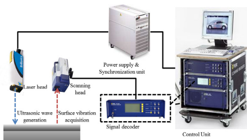
Fig. 1 Overall configuration of the proposed laser ultrasonic system
