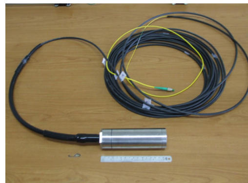
Fig. 9 Fiber optic pressure sensor package with stripped jacket.
