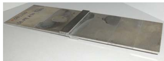
Fig. 7 Shaving shear-welded plate
