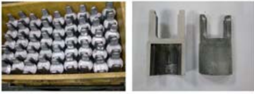
Fig.13 Final products after forging
