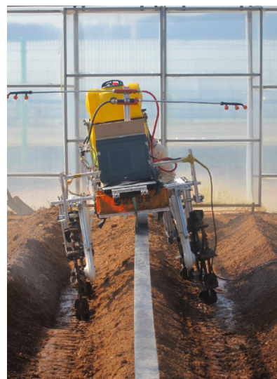
Figure 4. Snapshot of the sprayer on highly tilted pathway and uniformly leveled spraying boom.
