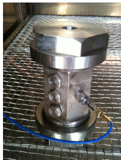
Fig. 3 The Pressure Bomb and Sample Mounting Used for Measuring of Pyrosensor Reaction
