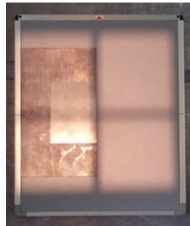
Fig. 4. Edge phantom placement and irradiation field set-up.
