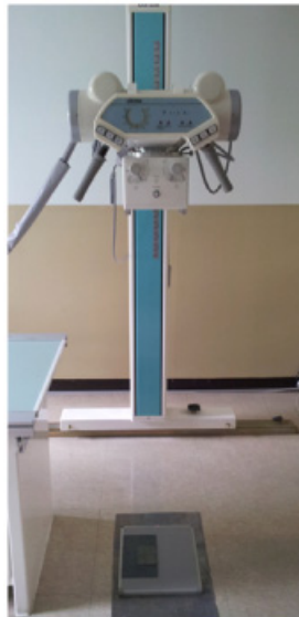
Fig. 3. Imaging set-up for MTF calculation.
