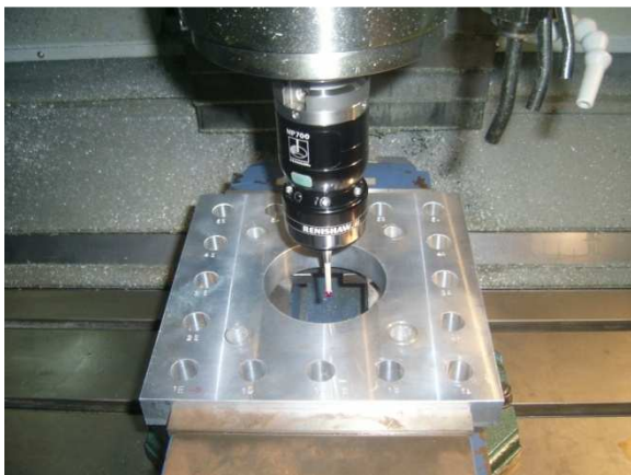
Fig. 8 Hole measurement on machine using Touch probe
