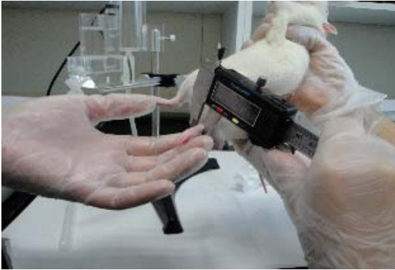
Scheme 2. A picture of the scene to measure the thickness of ankle joints of rats using Digital Caliper.
