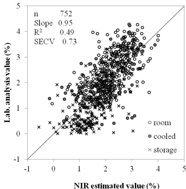
Figure 3. Sucrose content calibration (850-1040 nm)
