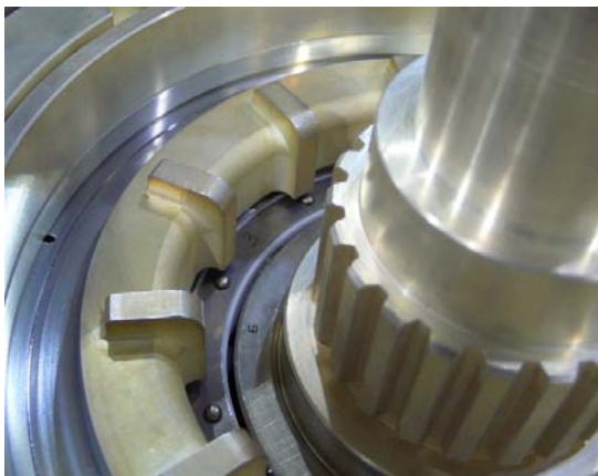
Fig. 3 Bearing supporter with vanes
