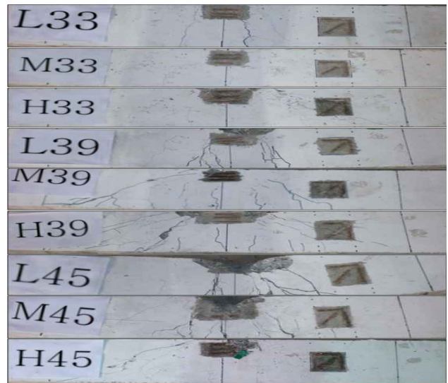
Figure 5. Crack pattern of test beams
