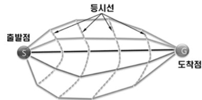
Fig. 4 Overview of the isochrone method
