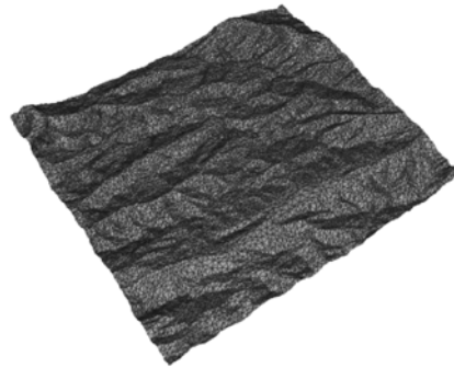
(b) Simplified triangular mesh (20,958 triangles)
