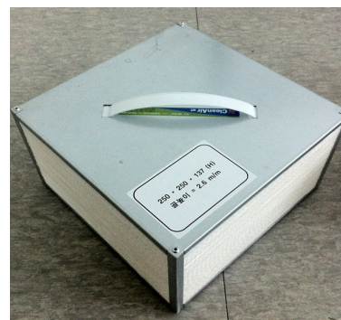
Fig. 1 Schematic and photo of paper heat exchanger.
