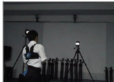
Figure 5. Subject with SPM in front of infrared light digital camera for motion capture
