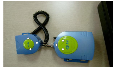
Figure 4. Six markers for motion capture attached to SPM
