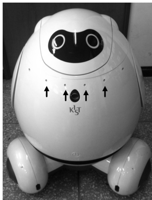
Fig. 4. Engkey robot with eight microphones (Four microphones indicated by arrows are used in this paper).
