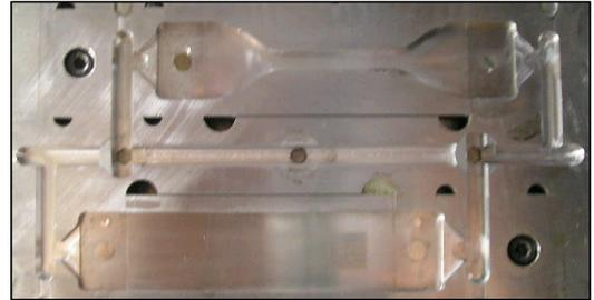
Fig. 2 A cavity shape of experimental mold
