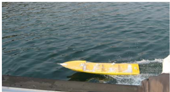
Fig. 14 At-sea model test of planing hull with air injection at the bottom
