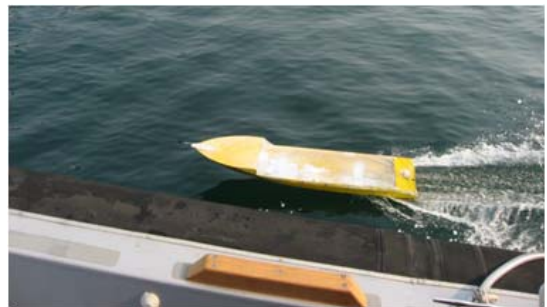
Fig. 13 At-sea model test of planing hull without air injection at the bottom
