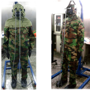
Fig. 8. The photograph of the thermal manikin test for NBC protective clothing
