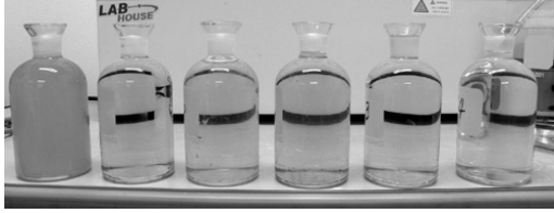
Figure 12. Chromaticity change by reactor. (Original water quality-MBR-Aeration tank-Setting tank-Treated water-Electrolysis treated water)
