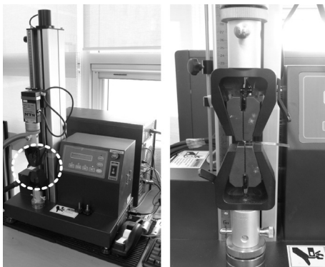
Fig. 10 Tensile tester for experimental of welding strength
