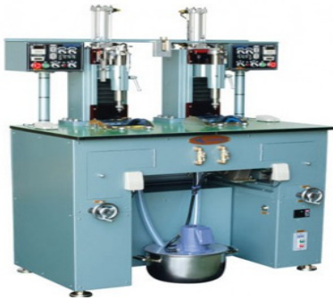
Fig. 3 Spherical center polishing machine
