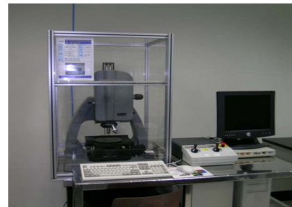
Fig. 6 Surface roughness measuring instrument(Newview5000)
