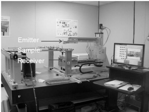
Fig. 2 THz TDS system for imaging and material parameter measurement
