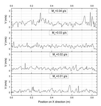
Fig. 6 Relationship between velocity magnitude on X-axis and air supply for D=12mm,  $\beta$ =0.60 at 17s
