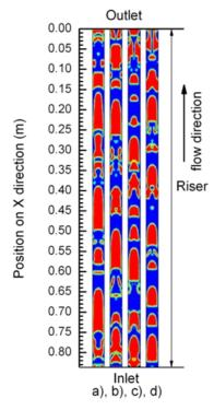
Fig. 7 Phase distribution in the riser with D=12 mm and  $\beta$ =0.60 at 17s, (a: M<sub>A</sub>=0.04 g/s; b: M<sub>A</sub>=0.03 g/s; c: M<sub>A</sub>=0.02 g/s; d: M<sub>A</sub>=0.01 g/s)
