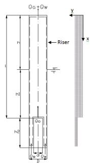
Fig. 2 Model of air-lift pump
