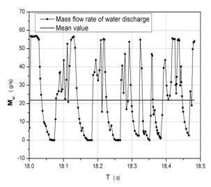
Fig. 4 Mass flow rate of water for D=12 mm,  $\beta$ =0.60, Ma=0.04 g/s
