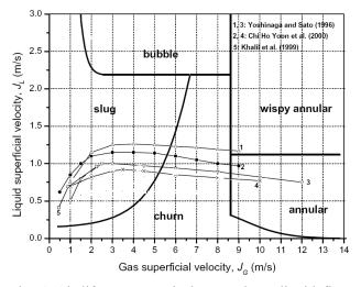
Fig. 1 Air-lift pump vertical upward gas-liquid flow regime map
