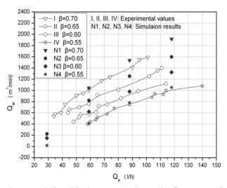
Fig. 5 Relationship between volumetric flow rate of water discharge and air supplied for D=12.00mm
