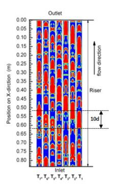
Fig. 3 Phase profiles in the riser from 16.766s to 17.385s for D=12mm, β=0.60, MA=0.04 g/s (red-gas slug, blue-liquid slug)
