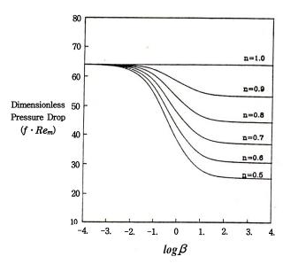
Fig. 2 Variation of dimensionless pressure drop with shear rate parameter  $(\beta)$  for shear-thinning fluids in a circular conduit
