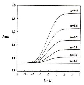
Fig. 3 Variation of Nusselt number (CHF) with shear rate parameter ( $\beta$ ) for shear-thinning fluids in a circular conduit
