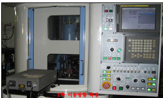
Fig. 2 Photo of positioning accuracy measurement system
