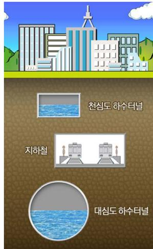
Fig. 9. Conceptual diagram of shallow and deep excavating type storages
