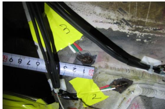
(b) position of the strain gauge grid  $S_L \geq 3$  mm
