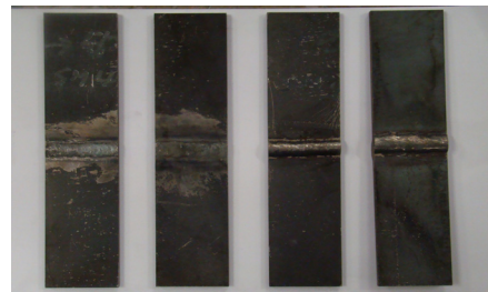
Fig. 3 Manufactured plate butt welding
