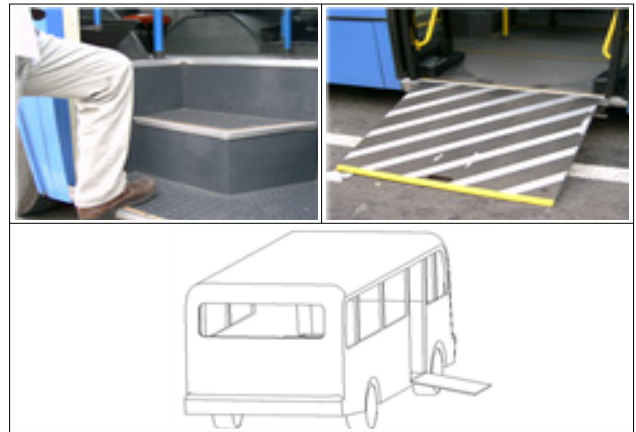
Fig. 12 Install the Ramp of the Gate
