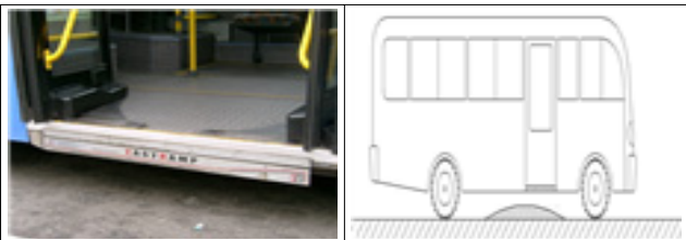
Fig. 10 Interference of the Gate and Speed Bumps
