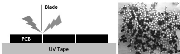
Fig. 9 Dicing Process of RFID Tag Package
