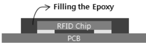
Fig. 6 Epoxy Molding for RFID Tag Package
