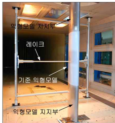
Fig. 1. Schematic of airfoil experiment in the KARI low-speed wind tunnel
