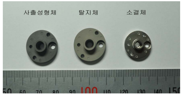
Fig. 7. Appearances of injection-molded, thermally debound and finally vacuum sintered fuze part
