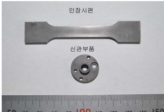
Fig. 6. Appearances of Injection-molded tensile specimen and fuze part
